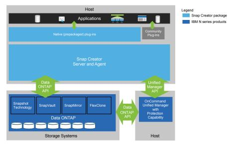
The IBM N series software products in the high-level diagram are optional; except for Snapshot technology, the other software products are not required for Snap Creator Framework to function.
